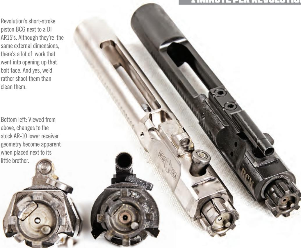
drops straight into an AR-15 upper. The bolt won't slide into an AR-15 barrel extension, giving the first clue that POF's engineers have managed to squeeze every last drop of performance out of the available real estate.
