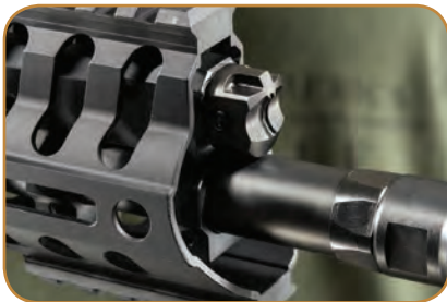
The Revolution's rifle-length gas system features a five-position adjustable gas block. Its location toward the end of the barrel increases dwell time and lowers the bolt carrier's velocity.
