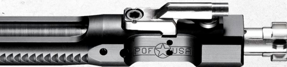
KEY-LOCK BOLT CARRIER GROUP The keylock design of this bolt carrier group is staked and bolted in, providing superior gas key stability. The carrier is Nitride heat treated for the ultimate in heat & pressure tolerance, lubricity, and wear resilience. Our bolt carrier groups feature a nickel plated bolt & extractor, and chrome plated firing pin. *For direct impingement rifles. Fits MIL-SPEC upper receivers.
