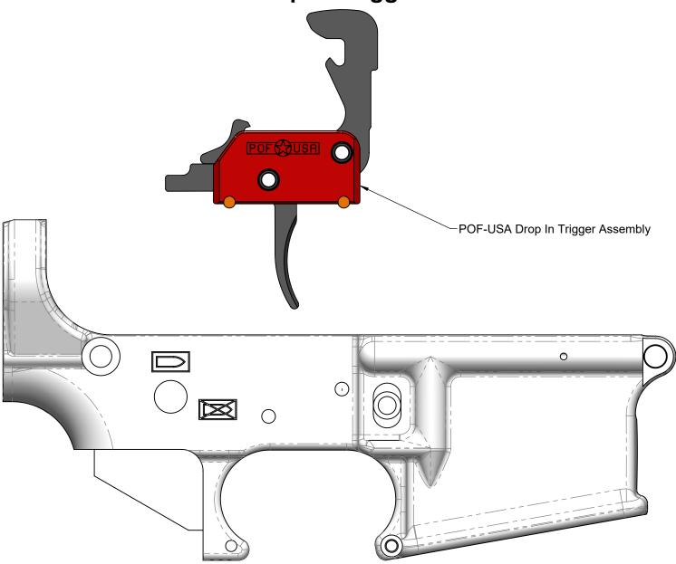
4. Remove the POF-USA Drop In Trigger Assembly. Install in reverse order from disassembly.
