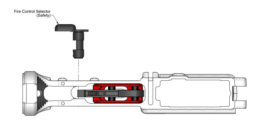
3. With the Trigger Assembly tilted back as instructed in step 2, remove the Fire Control Selector (Safety) from lower receiver.
