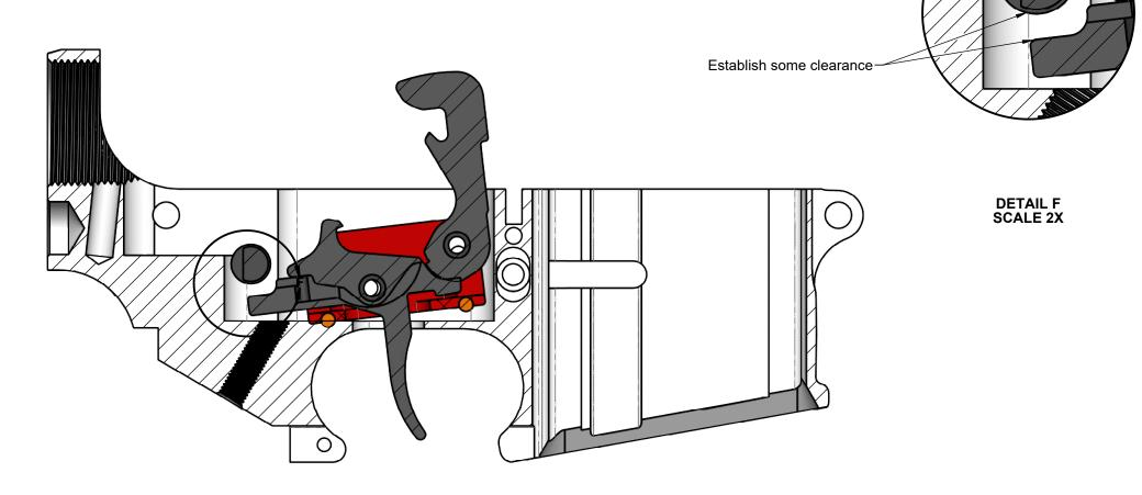
2a. Remove the Pistol Grip. With it should come the Selector Spring, and Selector Detent. This will allow the Selector to be moved at a later step.
