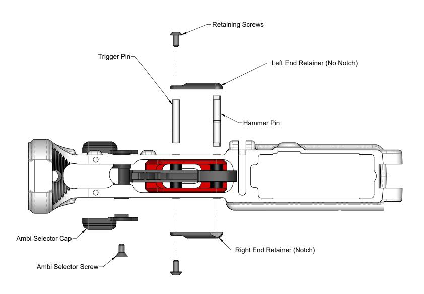
1a. Remove KNS Non-Rotating Pins by unscrewing retaining screws and removing end retainers. Then push out the hammer pin and trigger pin.
