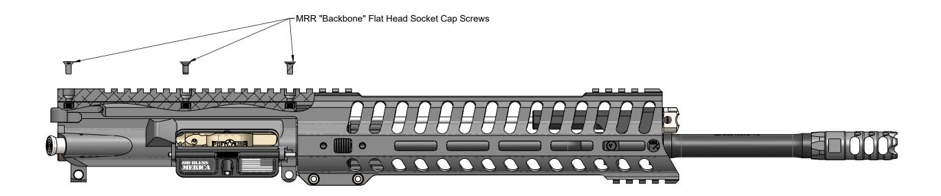
3. Using a IP20 Torx Plus or T20 Torx driver or wrench, remove the 8-32x3/8 "Backbone" Flat Head Socket Cap screws from the Edge MRR.
