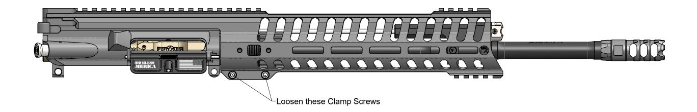
2. Using a 5/32 hex driver or hex wrench, loosen the 2 10-32x3/8 Socket Head Cap Screws that clamp the Edge MRR to the Heat Sink Barrel Nut.
