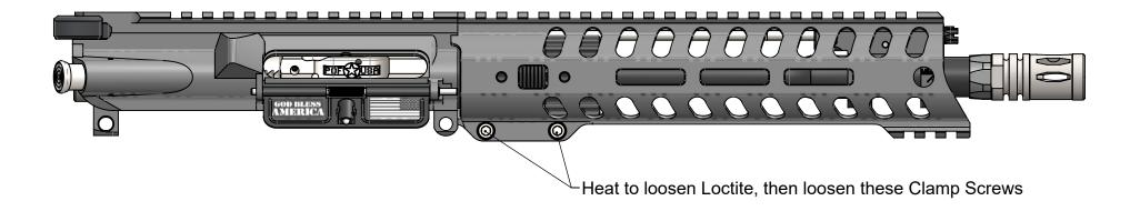
2. Heat up screws with blow dry or heat gun. The screws have loctite on them.
