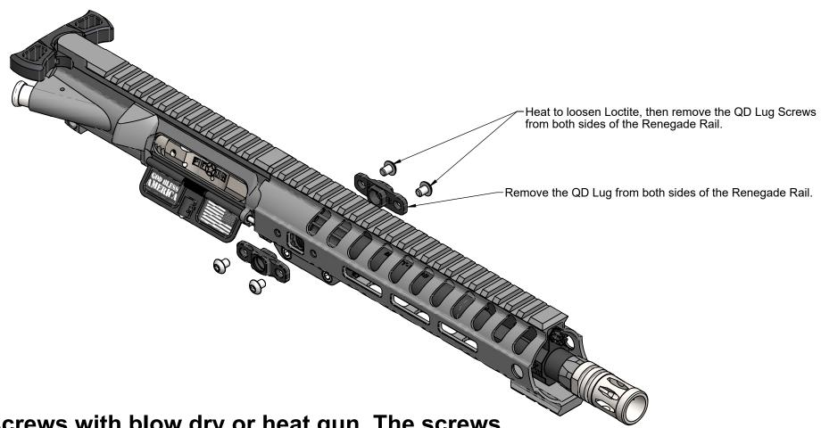
1. Heat up screws with blow dry or heat gun. The screws have loctite on them. Then, Using a IP25 Torx Plus or Torx T25 size driver, completely Remove the 4 total (2 per side) 10-32x1/4 QD Lug Screws, and the 2 QD Lugs they fasten, from each side of the Renegade Rail.
