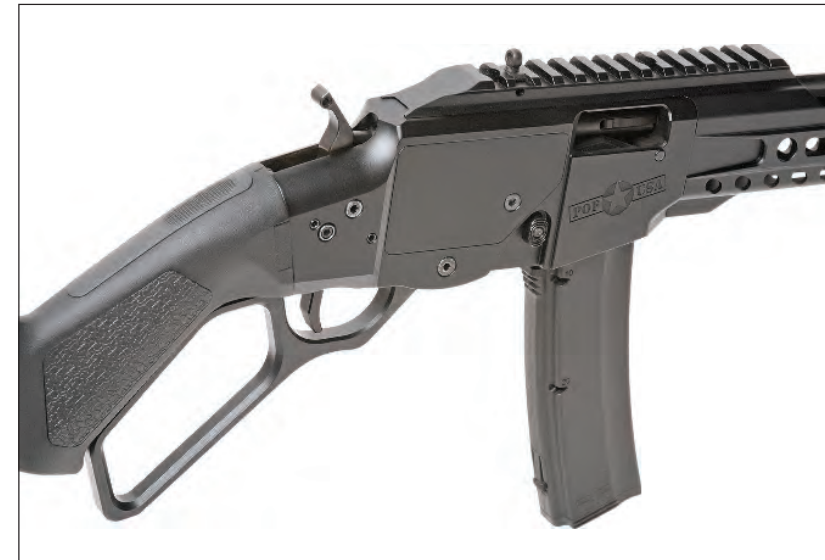
The beefy receiver has sort of a Winchester M1873 vibe to it with its angular lines. Note the ejection port, mag release button and optics rail with rear sight.
