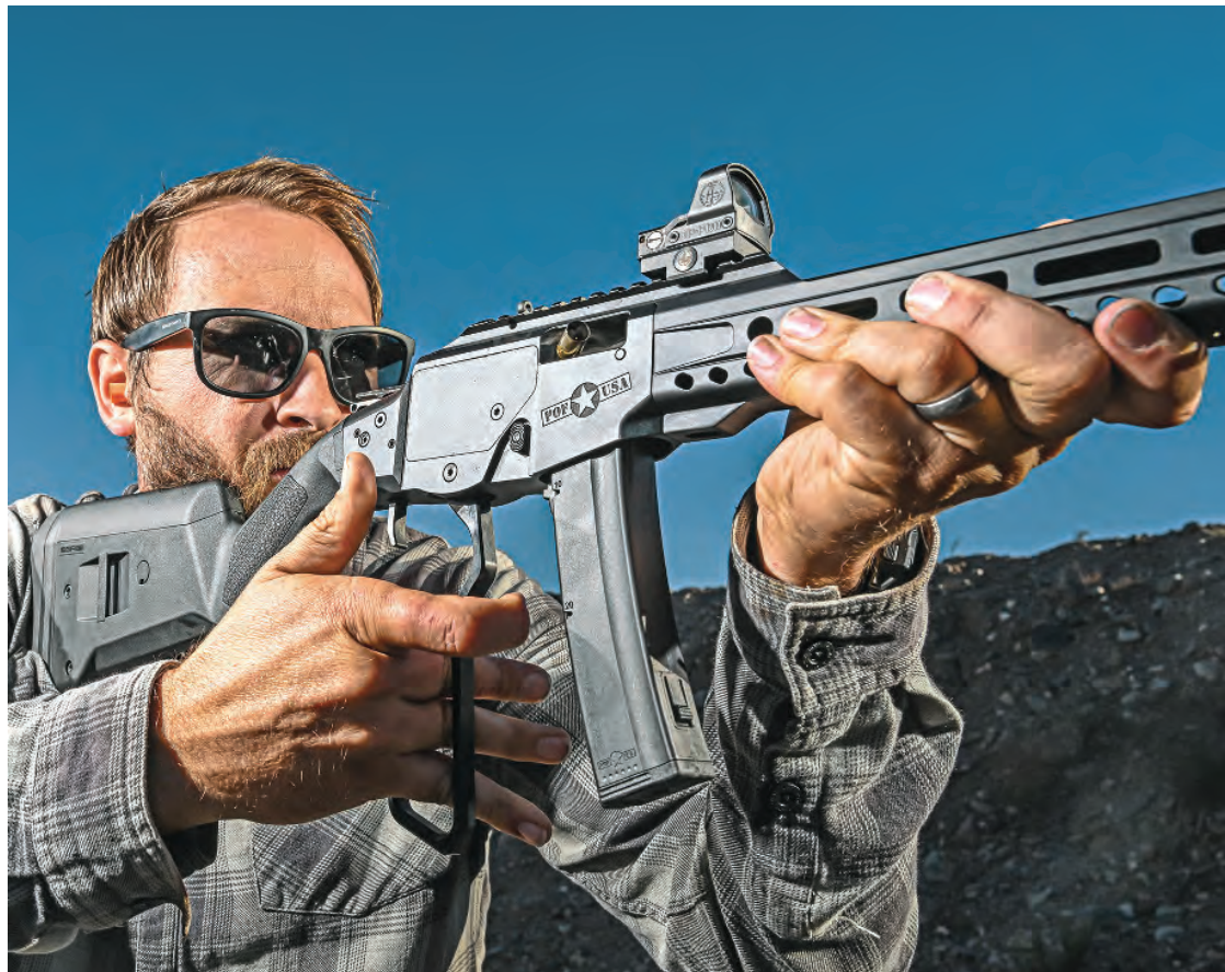
The action is run by a lever which forms the trigger guard and hand loop. The throw is short and does not require much effort. (Photo by Sean Utley)
