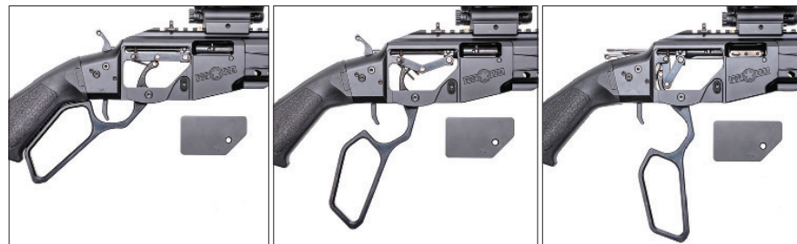
Removing the Tombstone's side plates exposes the unique linkage assembly. As the lever is pulled down, the linkage unlocks the bolt and pulls it rearward.
