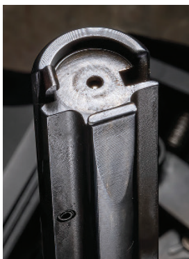
The bolt contains the firing pin within, an external extractor and a groove that allows the fixed ejector to pass through.
