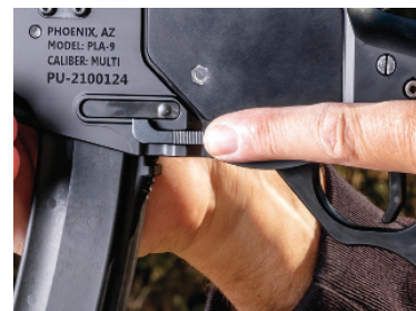
The magazine release is intuitive for users of the AR-15, however, the magazine is locked into place by a rear tab.
