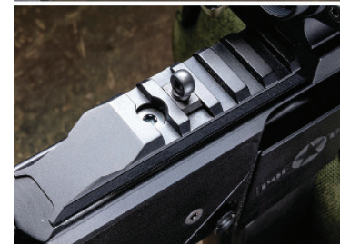
XS Sights' Ghost Ring sights are standard. While the post-aperture makes for a familiar sight setup, an optic works great, too.
