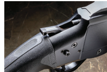
The crossbolt safety can be engaged when the hammer is placed in a half- or full-cock position.
