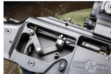
For inspections or maintenance, G&A recommends leaving one side plate in place to keep the linkage assembly intact.
