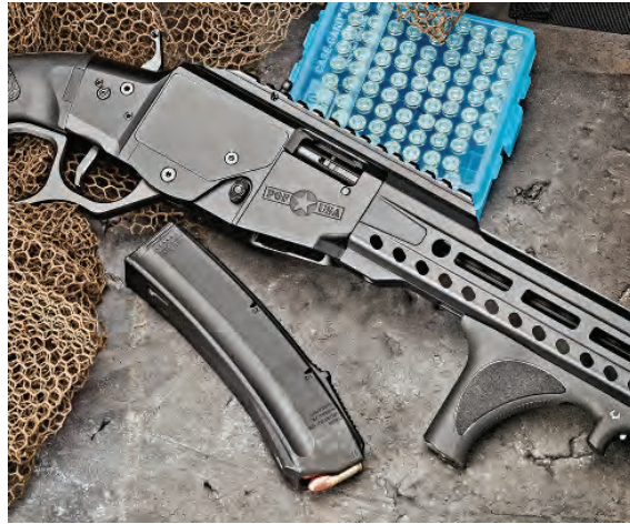
The carbine comes with one 20-round magazine. It's the same injection-molded magazine as used by POF's Phoenix semiautomatic pistol. The Tombstone's AR-style magazine release is ambidextrous.
