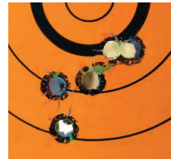
This 1.0-inch, five-shot group at 50 yards demonstrates the very good accuracy Joel achieved with the Tombstone lever action. The ammo was Hornady's 9mm 115-grain MonoFlex +P Handgun Hunter load.
