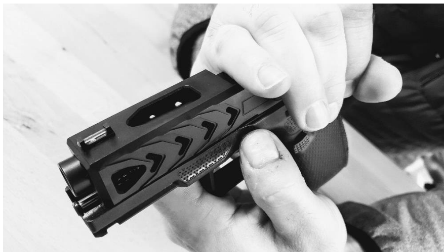
Figure 11. Pulling Down Slide Lock
