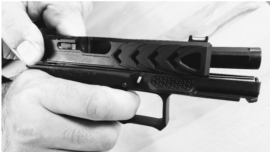
Figure 26. Proper Trigger Reset Test Technique
