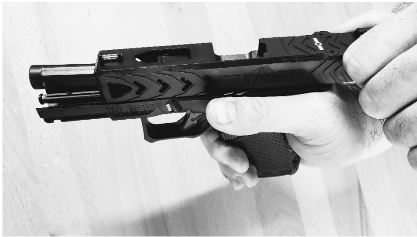
Figure 5. Locking Slide Back Via Slide Stop Lever
