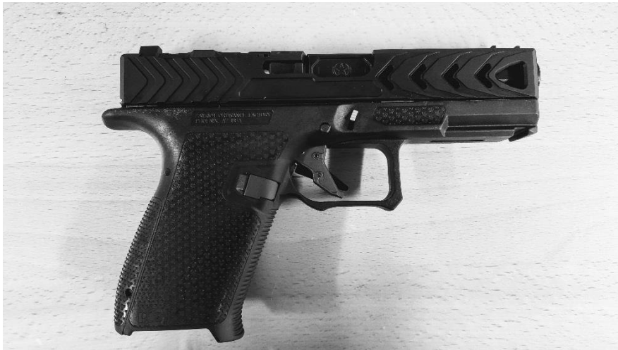
Figure 24. Rack Slide Back into Place
