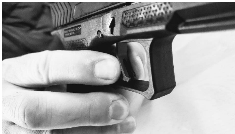
Figure 25. Proper Trigger safety Test Finger Placement
