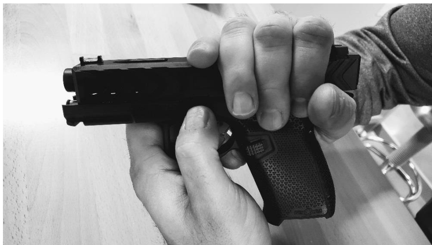
Figure 10. Properly Gripping P19 for Disassembly.
